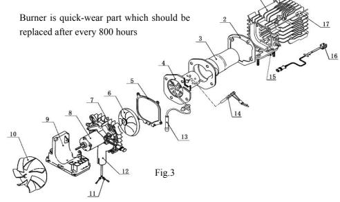
1-Heat exchanger 2-Gasket 3-Combustion pipe 4-Burner 5-Gasket 6-Combustion supporting fan blades 7-Bracket for fan motor 8-Fan motor 9-Controller 10-Blade wheel of heating fan 11-Fuel pump leading wire 12-Inlet of combustion supporting air 13-Fuel inlet pipe 14-Glow plug 15-Exhaust pipe vent 16-Overheat sensor 17-Insulating mat
