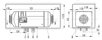
A-Inlet of heating air B-Outlet of heated air C-Inlet of combustion air D- Fuel inlet E-Exhaust outlet F- Non-interference area G-Installation surface H-Gasket
