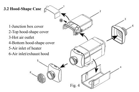
The structure of the hood-shape case is shown in Fig. 4. It consists of the top cover 2 (The junction box cover 1 can be fixed on 2), bottom cover 4, air inlet hood 6, air inlet of heater 5 and hot air outlet 3. They form an air heating passage. Blade wheel of heating fan (Fig.3-10) on the fan motor (the same for supporting combustion fan) sucks in cold air from the air inlet. The air is heated by the heat exchanger and sent out from the hot air outlet.
