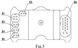
The connection parts are designed with such structures that wrong connection is made impossible.
