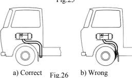
4.6.6 When the heat is working, the exhaust pipe is at high temperature. In installation, make sure to install it in far distance from plastic parts or other objects with poor thermal resistance of the vehicle body. The exhaust pipe shall be properly fixed. The exhaust vent shall be downwards, perpendicular to road surface with an angle of 90°±10°. To ensure such an angle, the fixing clamp for the exhaust pipe shall be within 150mm from the pipe end. (Fig. 27)
